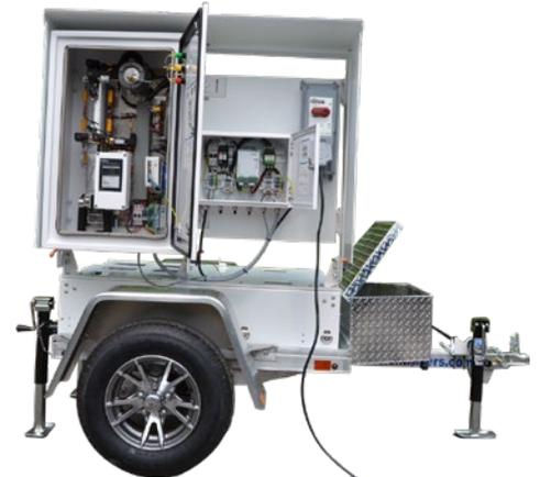
IP&L used Vaisala's Optimus™ Mobile multi-gas DGA Monitor, the OPT100 Mobile and Delta-X Research's Transformer Oil Analyst™ software with Monitor Watch™ to detect and identify faults on a suspect transformer. This was done without taking the transformer offline by using a mobile DGA online monitor and feeding its information to a cloud-based analytic software tool.
